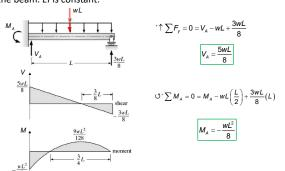
Analysis of statically indeterminate structures by the force method
