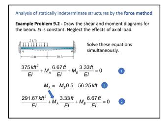
Analysis of statically indeterminate structures by the force method Example Problem 9.2 - Draw the shear and moment diagrams for the beam. El is constant. Neglect the effects of axial load. Solve these equations simultaneously.  $\frac{291.67 \, kft^2}{EI} + \left(-M_{\rm B}0.5 - 56.25 \, kft\right) \frac{3.33 \, ft}{EI} + M_{\rm B} \frac{6.67 \, ft}{EI} = 0$  $\frac{291.67 \, kft^2}{EI} + M_A \frac{3.33 \, ft}{EI} + M_B \frac{6.67 \, ft}{EI} = 0$
