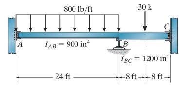
**Problem 10a-4** – Determine the moments at *A*, *B*, and *C*. Assume *A* and *C* are fixed, *B* is a roller, and *EI* is constant.
