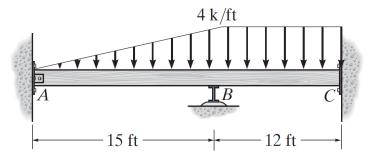
**Problem 10a-2** – Determine the moment at *B*. Assume the support at *A* is pinned, *B* is a roller, *C* is fixed, and *EI* is constant.
