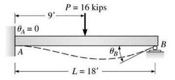
**Problem 10a-1** – Determine the moment at A. Assume the support at A is fixed and B is a roller. El is constant.
