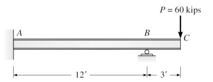
**Problem 9a-4** – Compute the reactions and draw the shear and moment curves for the following beam.
