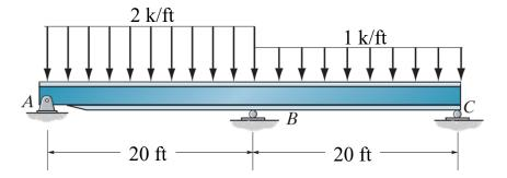
**Problem 9a-4** – Compute the reactions and draw the shear and moment curves for the following beam.
