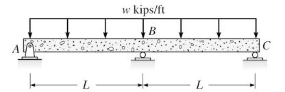
**Problem 9a-1** – Compute the reactions and draw the shear and moment curves for the following beam.
