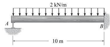
**Problem 9a-2** – Compute the reactions and draw the shear and moment curves for the following beam.
