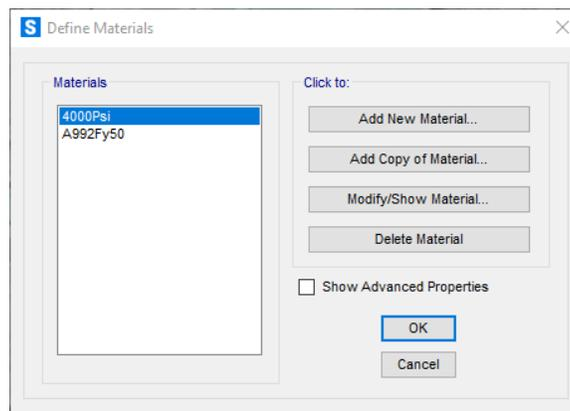
On this menu, you can change the properties of materials. Select the A992Fy50 (steel with a yield stress of 50 ksi) material in this example and click the **Modify/Show Material...** button.
