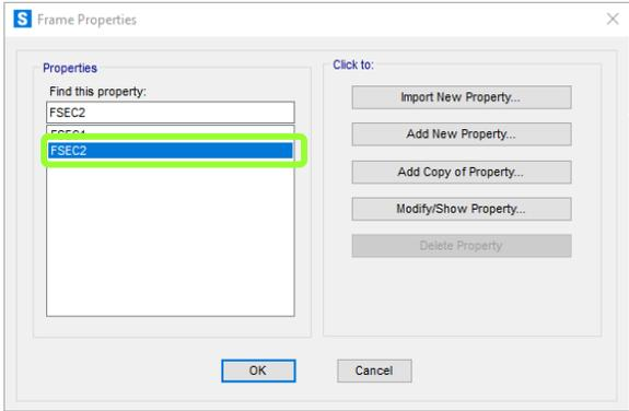
**Step 7: Assign Frame Sections** - To assign the frame properties of a structural element, select all frame elements with the pointer and click on the **Assign** menu at the top of the SAP2000 interface window, then click **Frame**, and then **Frame Sections**. You can assign the same section properties to multiple elements by selecting all the elements that share the same properties. Choose the **FSEC2** frame element from the **Assign Frame Sections** window and click **OK**.
