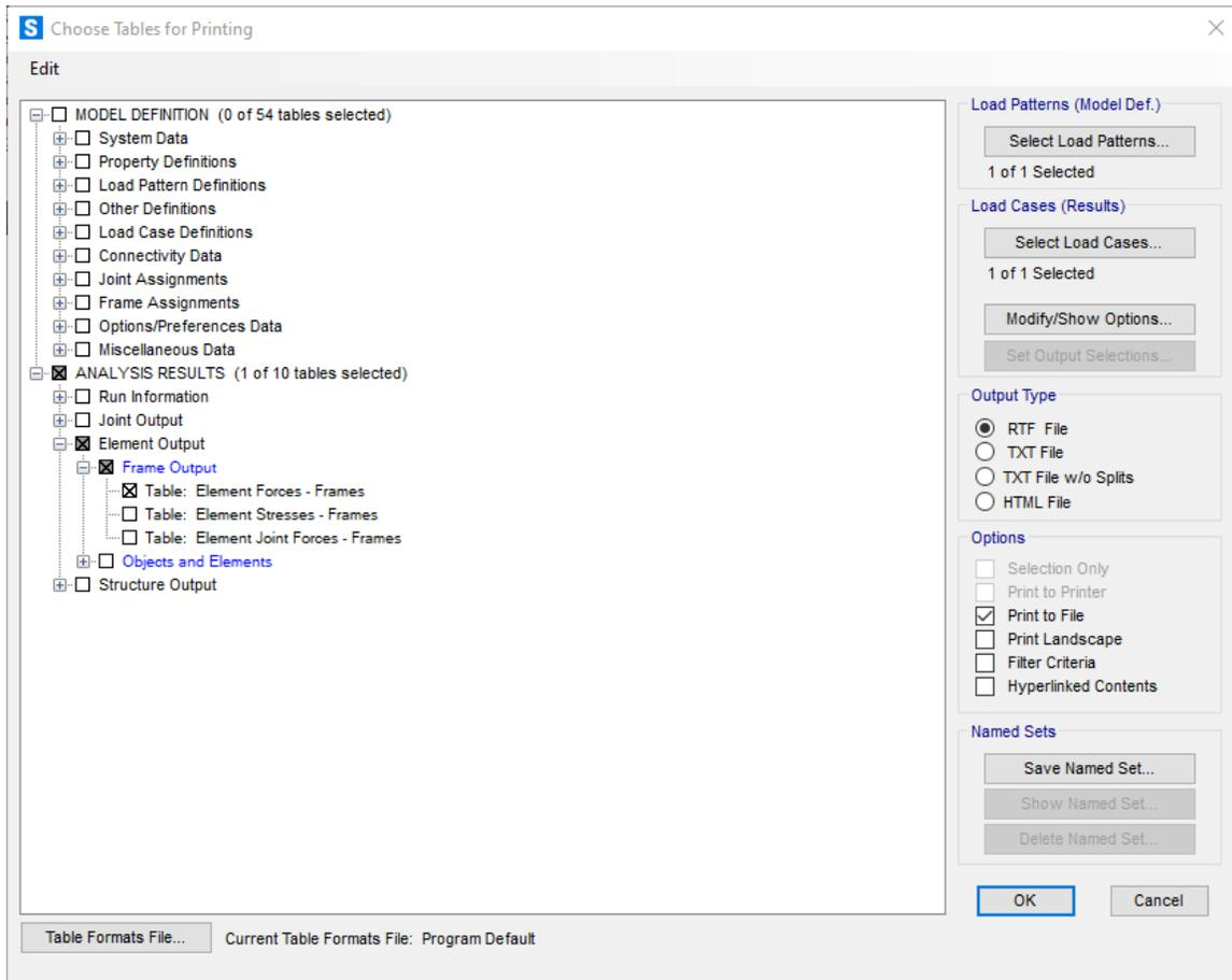
In this example, we want the shear forces and bending moments in the frame, so click on expand the **Element Output** item under the **ANALYSIS RESULTS** section, expand the **Frame Output** item, and then click on **Tables: Element Forces - Frames**. Also, click on the box **Print to File** and the **TXT file** button to define the file format. Click **OK** and define the name and location of the TXT file.
