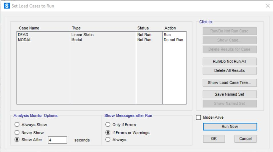
By default, there are two load cases: **DEAD** and **MODAL**. More load cases can be added, but only the **DEAD** load case is required for this example. Click on the **Run Now** button. If the analysis is successful, the **Analysis Complete** window is displayed and reports that the analysis is complete. Click **OK**, and the **Save Model File As** window is displayed.
