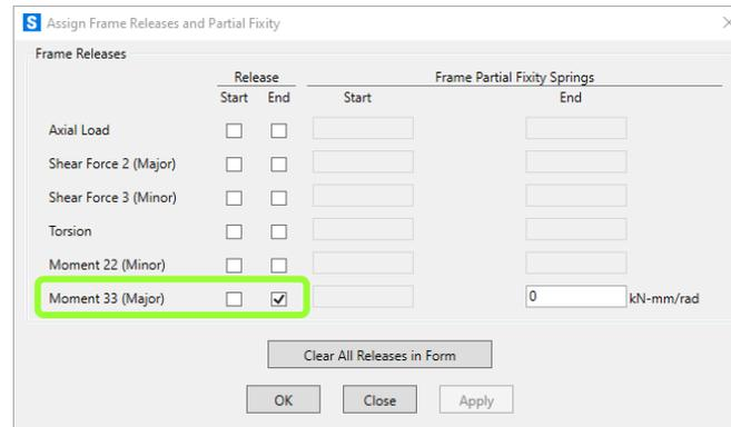
Check the box for Release End **Moment 33 (Major)**. The moment at the end of this element are zero. SAP2000 indicates that a release has been specified with a green dot and shows a break on the line.
