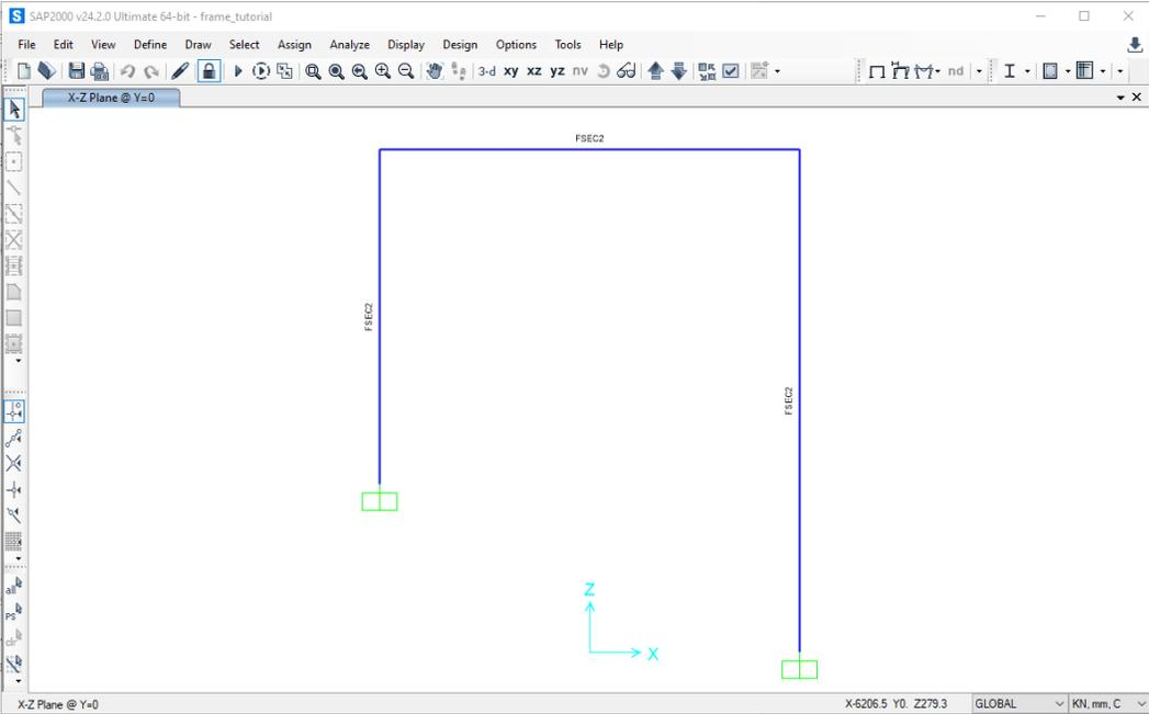
**Step 8: Run Analysis** - To analyze the model, press the Run Analysis button
