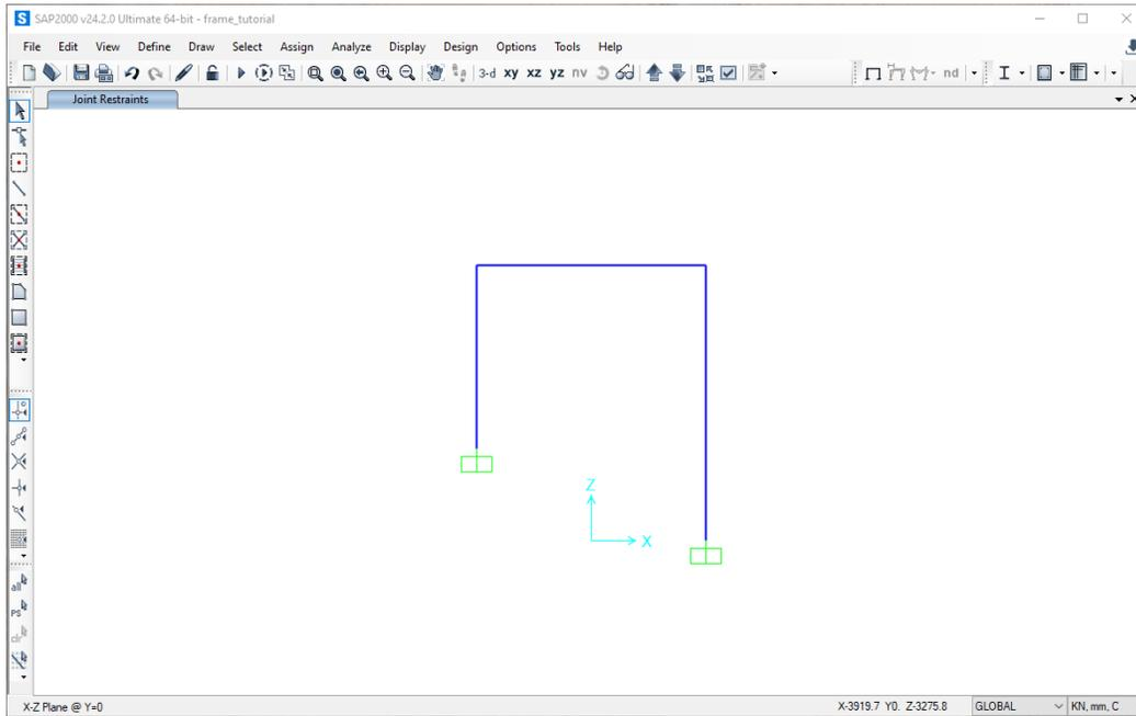
To model the pin connection at node *C*, select the frame element and click on **Assign, Frame, and Releases/Partial Fixity**. The following menu appears.
