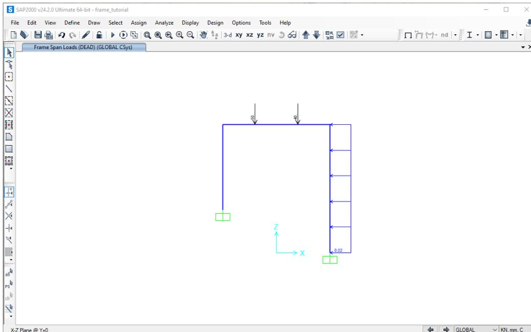
**Step 4: Set Analysis Options** - This example models the frame in the x-z plane. Click on the **Analyze** menu at the top of the SAP2000 interface window and then click **Set Analysis Options** to limit analysis to variables in the x-z plane. The **Analysis Options** menu appears as follows:
