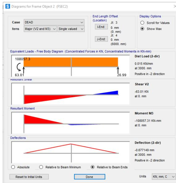
Drag the vertical slider along the element to see values on the loads, shear, moment, and deflection.
