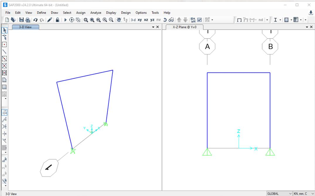
Since we do not need a 3-D view of the frame, click on the window label and delete the left-hand side window so that you have an **xz** view of the frame.
