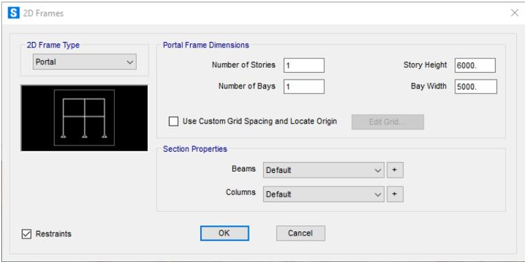
In this example, the frame has one bay of 5,000 mm (5 m) and a one-story height of 6,000 mm (6 m). Enter the values and click **OK**.
