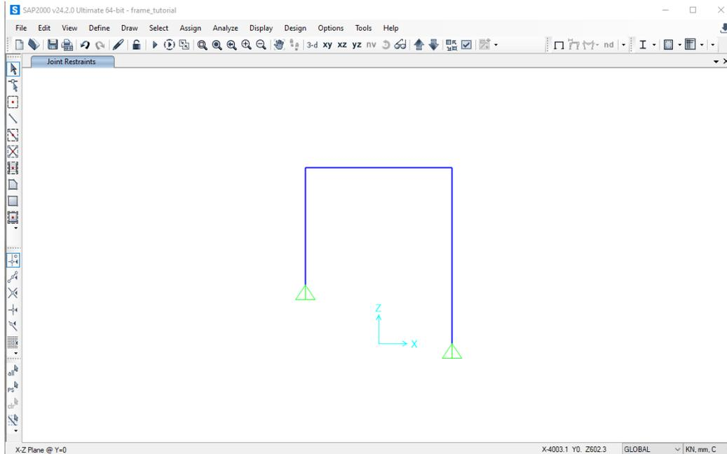
**Step 2: Define Structural Supports** - To define the location and type of structural support, select the support location by clicking on the joint with the pointer. A blue "X" should appear at the joint to indicate it is currently selected. Next, click on the **Assign** tab at the top of the SAP2000 interface, then click on **Joint**, and then the **Restraints ...** button on the bottom toolbar.
