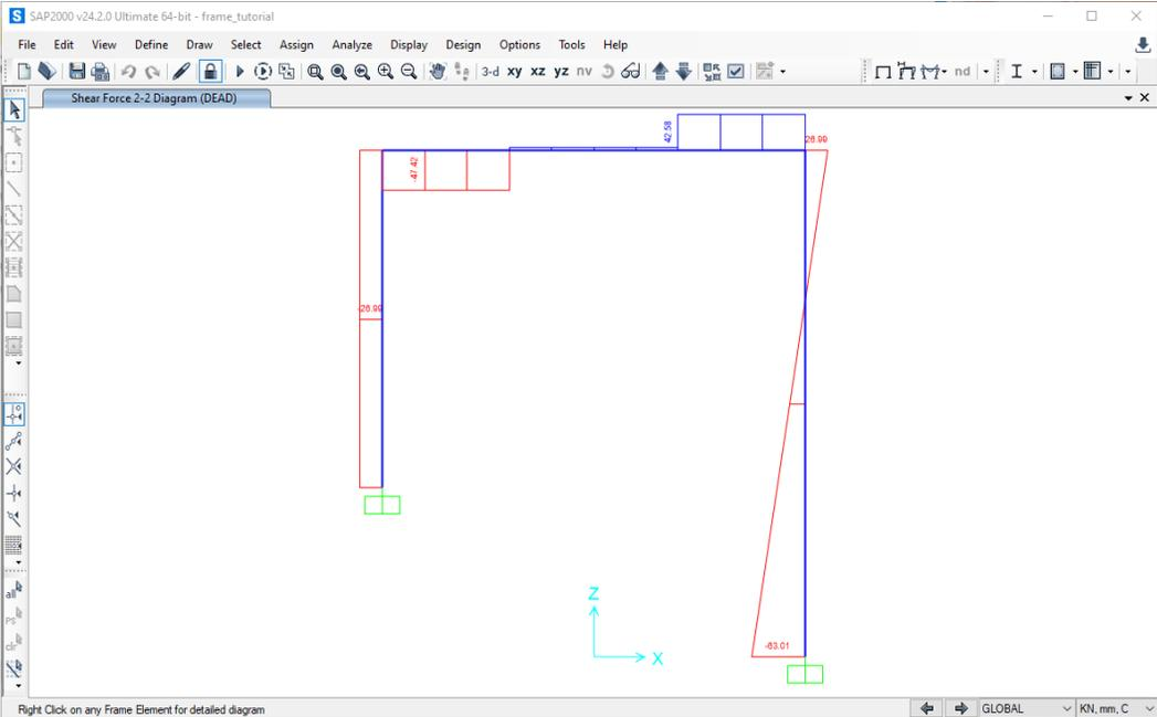
To view more detail about the forces along an element, click on the element in the SAP2000 interface and right-click. The **Diagram for Frame Object #** (FSEC2) window is displayed. Below are the results for each of the three elements in this example.
