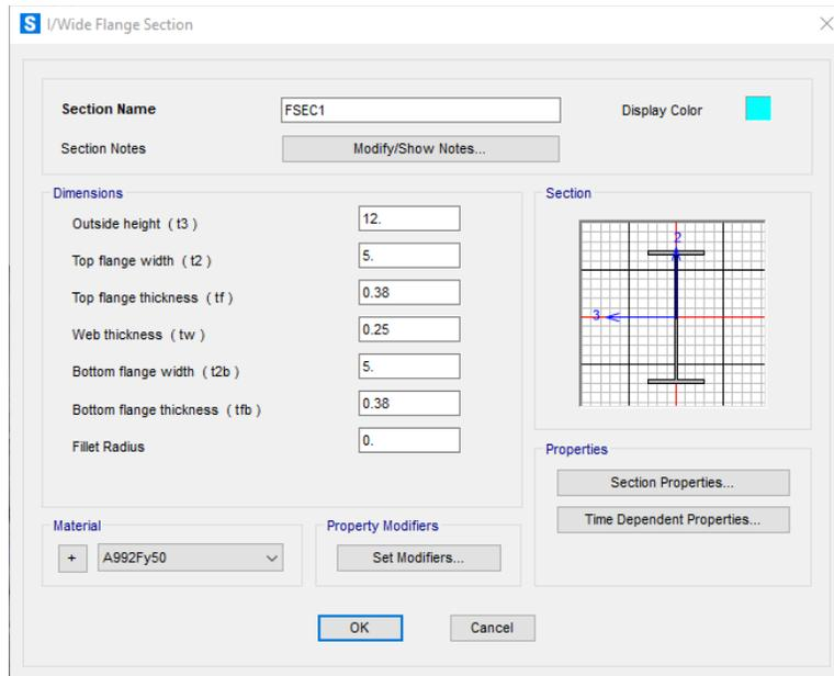
To define the material of this frame section, click on the **Material** pull-down menu and select our weightless material **A992Fy50**. Click **OK** to return to the **Frame Properties** window, then click **OK** again.
