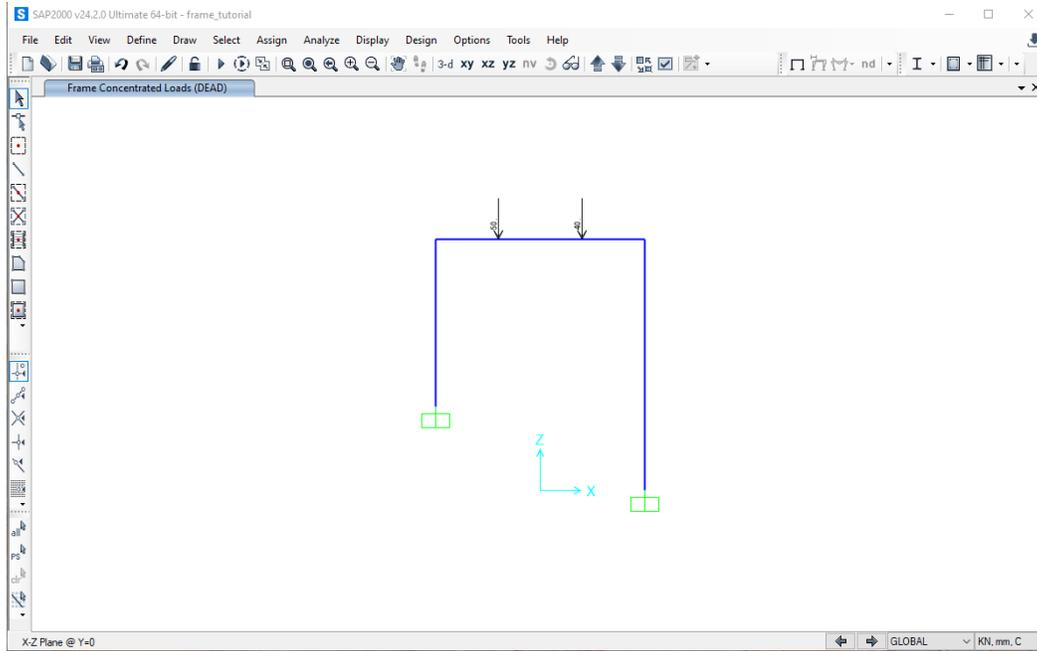
Next, click on the far right element and select **Assign, Frame Loads, and Distributed**. The following menu should be displayed. In this example, the distributed load is in the negative local x-direction and has a value of 0.015 kN/mm (15 kN/m). Enter these values into the menu and click **OK**.
