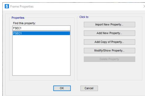
The default Frame Section label is **FSEC1**. To change the properties of the frame section, click on the **Modify/Show Property...** button. The **I/Wide Flange Section** window is displayed.
