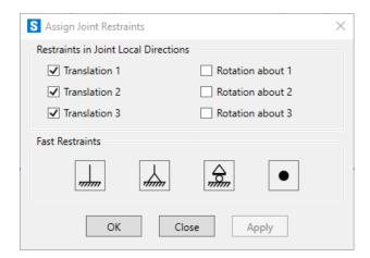
The **Assign Joint Restraints** menu appears as shown. Usually, the directions **1**, **2**, and **3** listed on the menu correspond to the x, y, and z directions. The Fast Restraints buttons may be used for most problems when working on two-dimensional structures. If the support conditions for your problem are not listed in the **Fast Restraints** section of the menu, you should select the appropriate combination of restraints.
