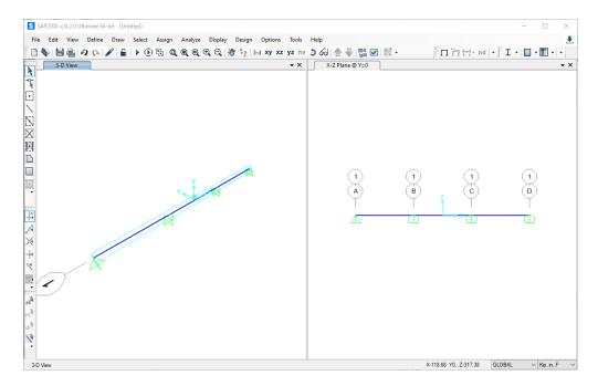
Since we do not need a 3-D view of the beam, click on the window label and delete the left-hand side window so that you have an **xz** view of the beam.
