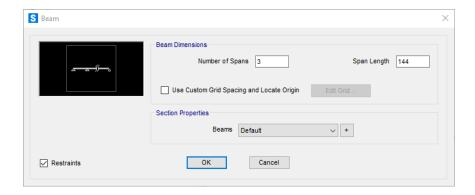
The SAP2000 interface displays the beam's geometry. By default, the left support is a pin, and the remaining supports are rollers.
