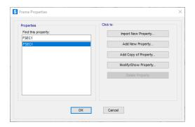
The default Frame Section label is **FSEC1**. To change the frame section's properties, click the Modify/Show Property... button. The I/Wide Flange Section window will then be displayed.
