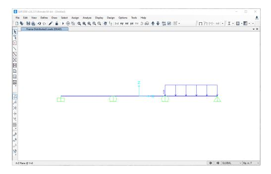
The point loads are not deleted; they are currently not displayed. Select Display, Show Object Load Assigns, Frame, and then OK to see all frame loads.
