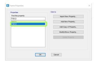
**Step 7: Assign Frame Sections** - To assign the frame properties of a structural element, select all beam elements with the pointer and click on the **Assign** menu at the top of the SAP2000 interface window, then click **Frame**, and then **Frame Sections**. You can assign the same section properties to multiple elements by selecting all the elements that share the same properties. Choose the **FSEC2** frame element from the **Assign Frame Sections** window and click **OK**.
