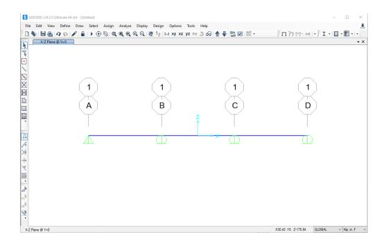
**Step 2: Define Structural Supports** - To define the location and type of structural support, select the support location by clicking on the joint with the pointer. A blue "X" should appear at the joint to indicate it is currently selected. Next, click on the **Assign** tab at the top of the SAP2000 interface, then click the Joint and the **Restraints** ... button on the bottom toolbar.
