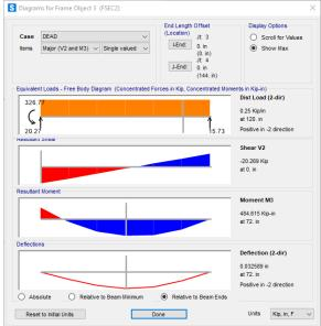
You can drag the vertical slider along the element to see the values for the loads, shear, moment, and deflection.
