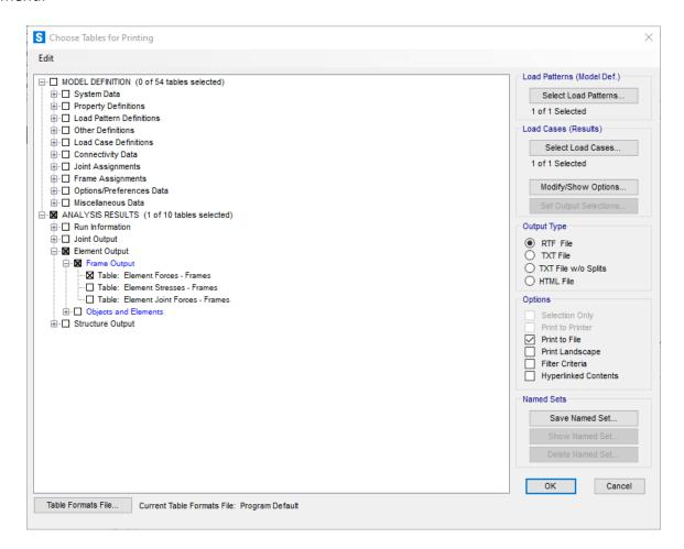
In this example, all we require is the mon the beam, so click on expand the **Element Output** item under the **ANALYSIS RESULTS** section, expand the **Frame Output** item, and then click on **Tables: Element Forces - Frames**. Also, click on the Print to File box and the **TXT file** button to define the file format. Click **OK** and define the name and location of the TXT file.
