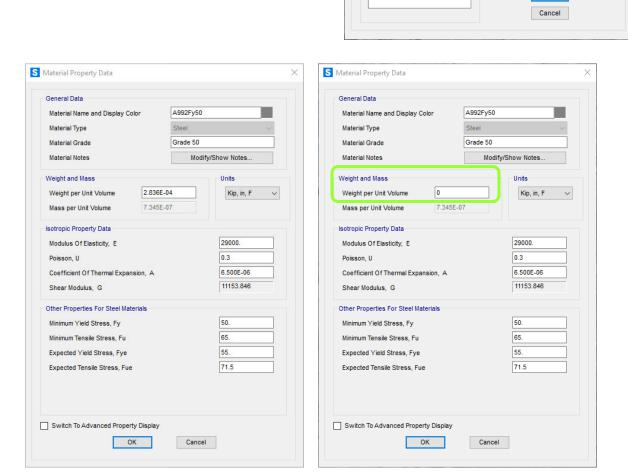
Change the value in the **Weight per unit Volume** input field to zero. Click **OK** to return to the **Define Materials** window, then click **OK** again. Now, we have a material named **A992Fy50** that does not weight volume. For this example problem, the default values for the Mass per unit Volume, Modulus of elasticity, Poisson's ratio, and the Coefficient of Thermal Expansion can be
