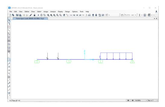
**Step 4: Set Analysis Options** - This example models the beam in the x-z plane. Click on the **Analyze** menu at the top of the SAP2000 interface window and then click **Set Analysis Options** to limit analysis to variables in the x-z plane. The **Analysis Options** menu appears as follows:
