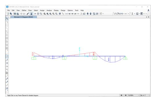
To view more detail about the forces along an element, click on the element in the SAP2000 interface and right-click. The **Diagram for Frame Object** # (FSEC2) window is displayed. Below are the results for each of the three elements in this example.
