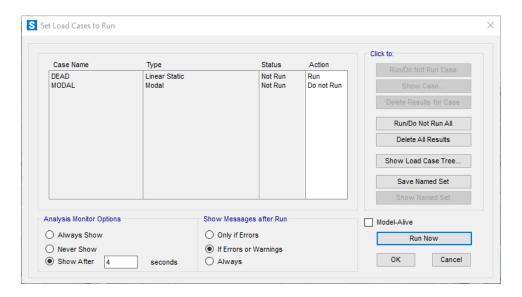
By default, there are two load cases: **DEAD** and **MODAL**. More load cases can be added, but only the **DEAD** load case is required for this example. Click on the **Run Now** button. If the analysis is successful, the **Analysis Complete** window is displayed and reports that the analysis is complete. Click **OK**, and the **Save Model File As** window is displayed.
