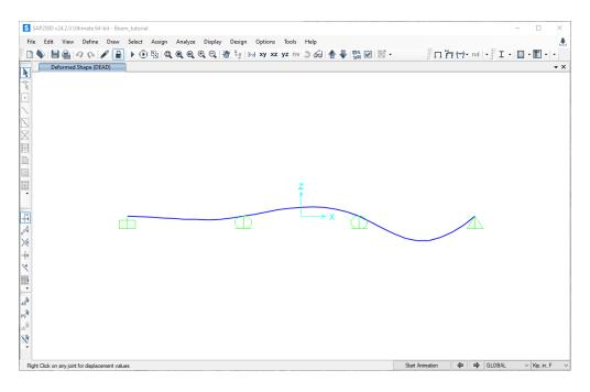
**Step 9: Print Beam Forces** - To get a quick feel for the relative magnitude of the forces in the beam, click on the **Show Forces/Stresses** pull-down menu to at the top of the SAP2000 interface, select **Frames/Cables/Tendons...**, and the **Display Frame Forces/Stresses** menu is displayed.
