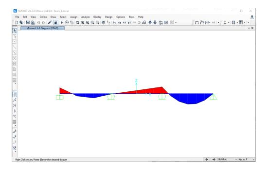
The default view is the **Fill Diagram**, which displays the relative magnitude of the moments. Negative bending moments are in red, and positive ones are in **blue**.
