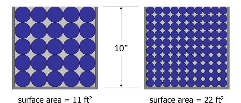
Use the largest NMAS you are allowed to in order to minimize the surface area per cubic yard of concrete
