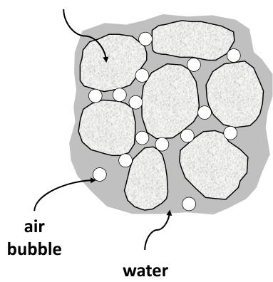
Air entrainment adds lubrication without adding additional water
