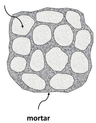
Need enough mortar to keep all the gravel particles apart.
