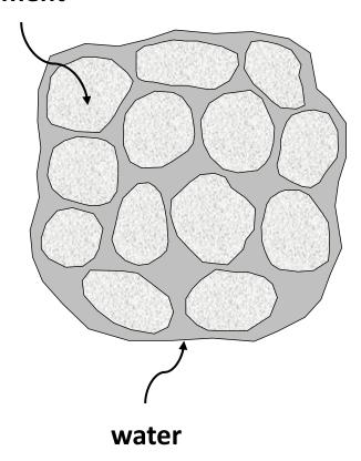
Need enough mixing water to lubricate all the cement grains
