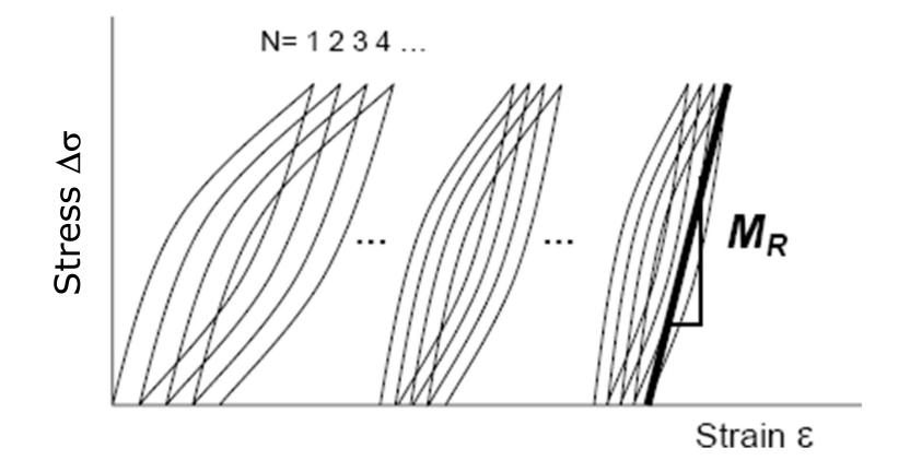
The resilient modulus test is typically run at 3 to 5 different confining pressures and, for each confining pressure, 3 to 5 different axial loads are applied. At the end of the test, the bulk stress can be calculated  $(\theta = \sigma_{axial} + 2\sigma_{lateral})$  and the results plotted as a function of the bulk stress. This allows the designer to choose a resilient modulus corresponding to the stresses present in the pavement system.
