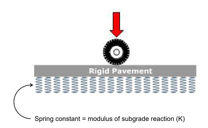
The modulus of subgrade reaction is measured in the field by conducting a *plate load test*, which measures the force needed to push a circular metal plate into the surface of the roadbed material.
