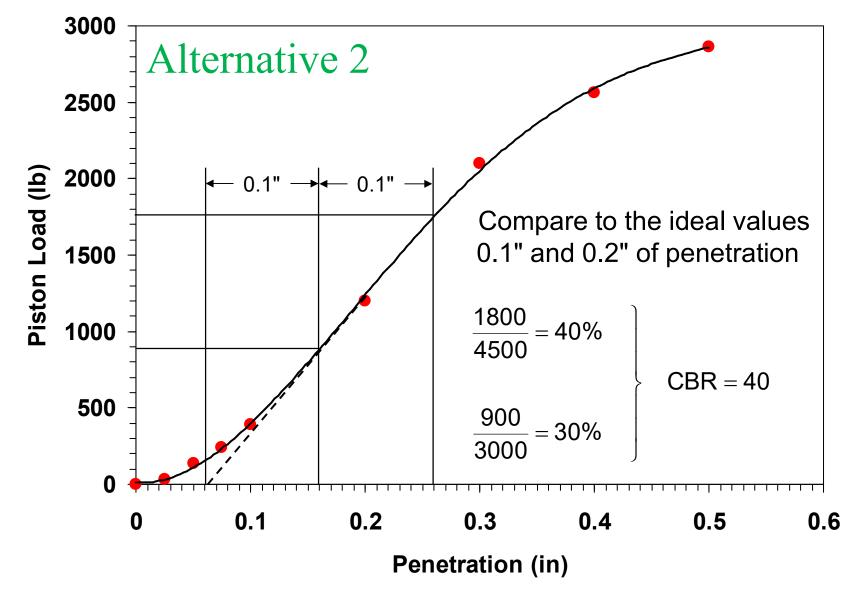
The CBR test can also be conducted in the field by jacking against the bumper of a truck and measuring the penetration of the plunger against a reference beam anchored outside of the zone of influence of the plunger (typically an area 3-4 ft in diameter).
