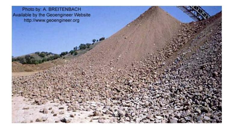
Aggregate sampling is the process of taking a sample of aggregate that is truly representative of the nature and condition of the aggregate in the stockpile. The size of the **field sample** is large to ensure that it is truly representative. Special effort must be made to ensure that the sample is not skewed by the effects of segregation.
