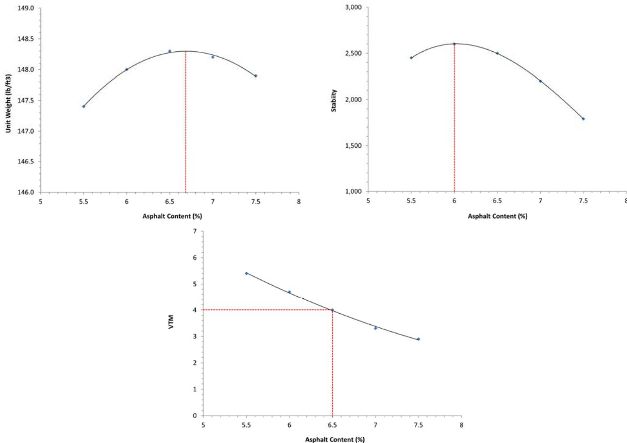
$$AC = \frac{\text{Max Density} + \text{Max Stability} + \text{4% Air Voids}}{3} = \underline{\underline{6.4\%}}$$
