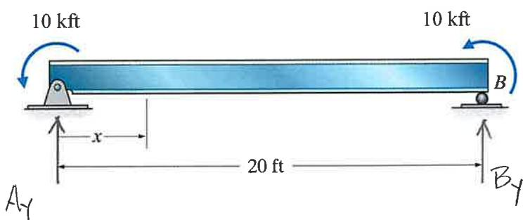
$$\begin{aligned} \textcircled{+} \sum M_B &= 0 \\ &= 10\text{kft} + 10\text{kft} - A_y(20\text{ft}) \\ A_y &= 1\text{k} \end{aligned}$$
