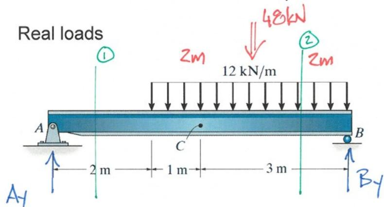
$$\text{At } B: \sum M_B = 0 = 48\text{kN}(2\text{m}) - A_y(6\text{m}) \quad \underline{A_y = 16\text{kN}}$$
