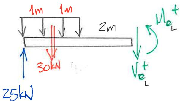
$$\text{At } \sum M_{\text{cut}} = 0 = M_{D_L} + 30 \text{ kN}(3\text{m}) - 25 \text{ kN}(4\text{m})$$
