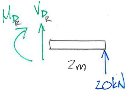
$$\text{At } \sum M_{\text{cut}} = 0 = -M_{D_R} + 20 \text{ kN}(2\text{m})$$
