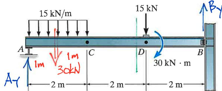
$$\text{At } B: \sum M_B = 0 = -30 \text{ kN}\cdot\text{m} + 15 \text{ kN}(2\text{m}) + 30 \text{ kN}(5') - A_y(6\text{m})$$
