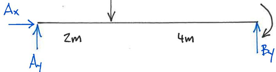
$$+\sum M_B = 0 = -20 \text{ kNm} + 6 \text{ kN}(4\text{m}) - A_y(6\text{m})$$
