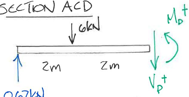
$$+\sum M_{\text{cut}} = 0 = M_D + 6 \text{ kN}(2\text{m}) - 0.67 \text{ kN}(4\text{m})$$
