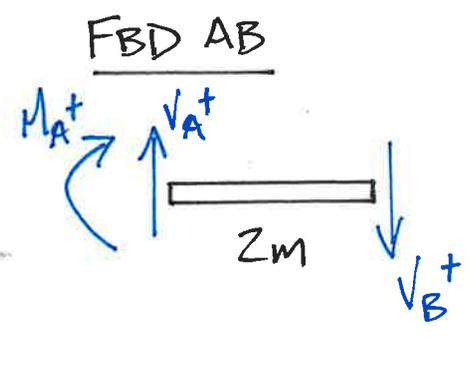
$$\begin{aligned} \sum M_A = 0 &= -M_A - V_B(2m) & \underline{M_A = 20kNm} \\ \sum F_y = 0 &= V_A - V_B & \underline{V_A = -10kN} \end{aligned}$$
