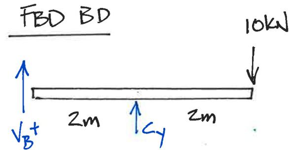
$$\begin{aligned} \sum M_C = 0 &= -V_B(2m) - 10kN(2m) & \underline{V_B = -10kN} \\ \sum F_y = 0 &= V_B + C_y - 10kN & \underline{C_y = 20kN} \end{aligned}$$
