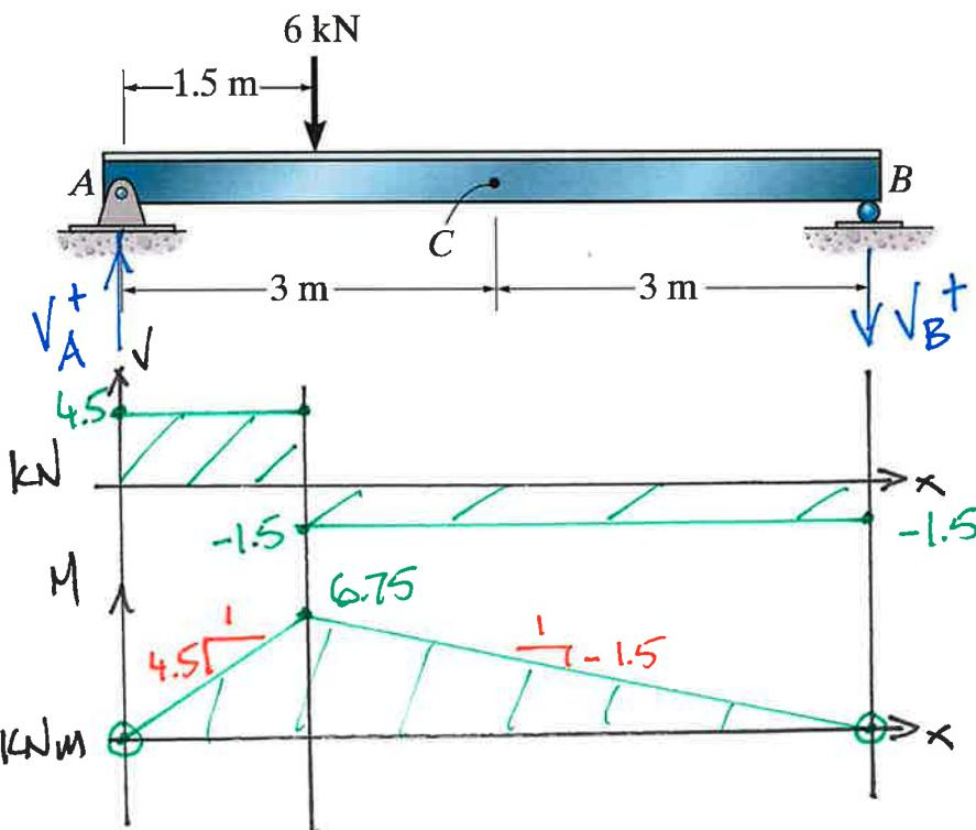
$$\begin{aligned} \text{At } B: \sum M_B = 0 &= 6\text{kN}(4.5\text{m}) - V_A(6\text{m}) & V_A = 4.5\text{kN} \\ +\uparrow \sum F_y = 0 &= V_A - V_B - 6\text{kN} & V_B = -1.5\text{kN} \end{aligned}$$
