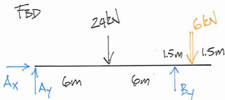
$$\rightarrow \sum M_A = 0 = -24 \text{ kN}(6\text{m}) - 6 \text{ kN}(13.5\text{m}) + B_y(12\text{m})$$
