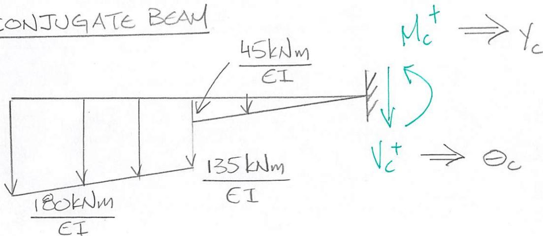
**Example 7b-5:** Use the conjugate beam method to determine the slope and displacement at point C.
