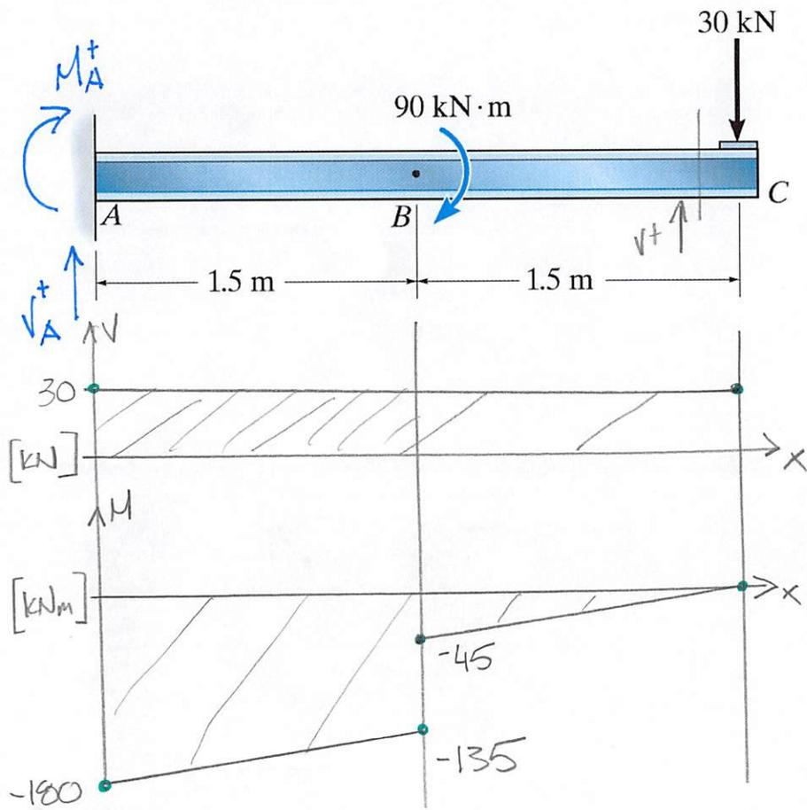
$$\sum M_A = 0 = -M_A - 90 \text{ kN}\cdot\text{m} - 30 \text{ kN}(3 \text{ m})$$
