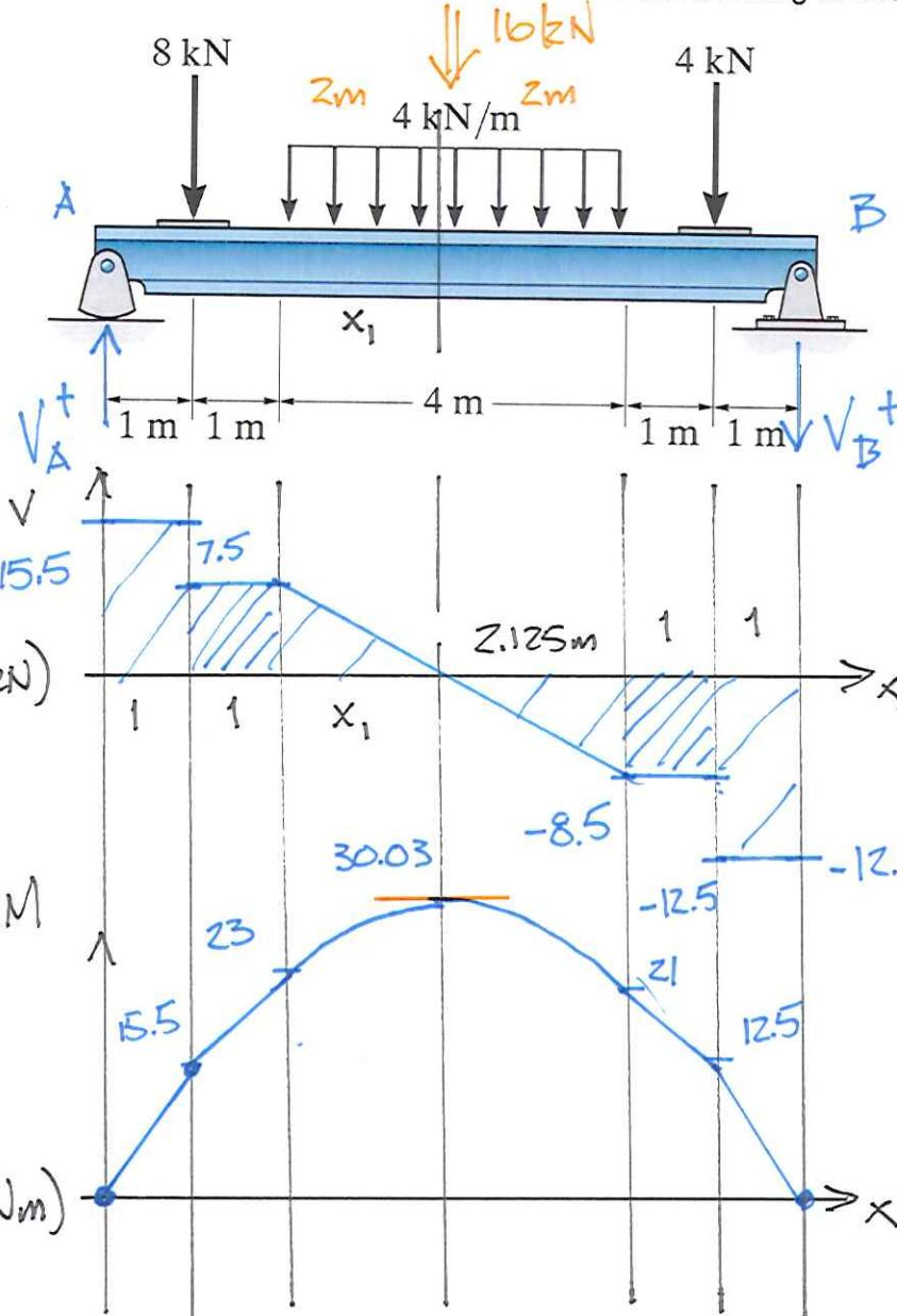
$$\begin{aligned} \text{At } B: \sum M_B = 0 &= 4 \text{ kN}(1 \text{ m}) + 16 \text{ kN}(4 \text{ m}) + 8 \text{ kN}(7 \text{ m}) \\ -V_A(8 \text{ m}) &\quad V_A = 15.5 \text{ kN} \\ +\uparrow \sum F_y = 0 &= V_A - V_B - 8 \text{ kN} - 16 \text{ kN} - 4 \text{ kN} \\ V_B = -12.5 \text{ kN} & \end{aligned}$$
