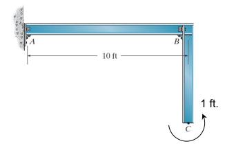
**Example 8c-3**: Determine the slope at point A. Assume E = 29,000 ksi.
