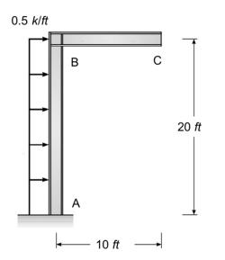
**Example 8c-2**: Determine the horizontal displacement at point C. Assume *EI* is constant.
