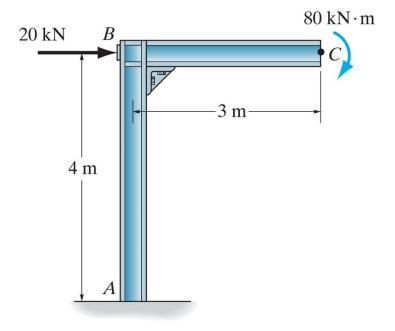
**Example 8c-6**: Compute the vertical displacement at point *C* on the frame shown. Include only the effects of the bending moment in your virtual work equations.
