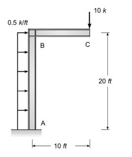
**Example 8c-1**: Compute the vertical deflection and rotation at point C on the frame shown. Include only the effects of the bending moment in your virtual work equations. Assume E = 29,000 ksi and  $I = 1,000 \text{ in}^4$ .
