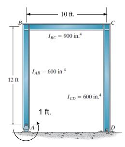
**Example 8c-4**: Compute the horizontal deflection at point *B* on the frame shown. Include only the effects of the bending moment in your virtual work equations.
