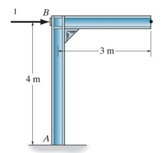
**Example 8c-5**: Compute the slope at point *C* on the frame shown. Include only the effects of the bending moment in your virtual work equations.
