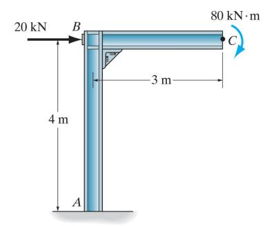
**Example 8c-4**: Compute the horizontal deflection at point *B* on the frame shown. Include only the effects of the bending moment in your virtual work equations.
