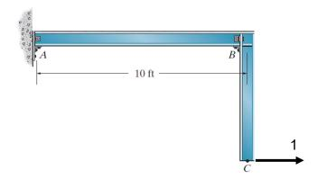
**Example 8c-2**: Determine the horizontal displacement at point C. Assume *EI* is constant.
