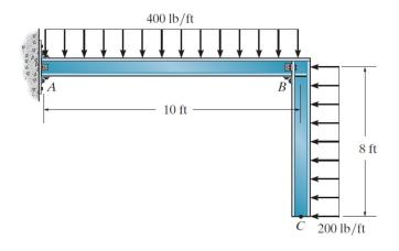
**Example 8c-2**: Determine the horizontal displacement at point C. Assume *EI* is constant.
