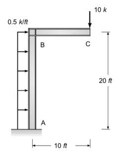
**Example 8c-1**: Compute the vertical deflection and rotation at point C on the frame shown. Include only the effects of the bending moment in your virtual work equations. Assume E = 29,000 ksi and  $I = 1,000 \text{ in}^4$ .
