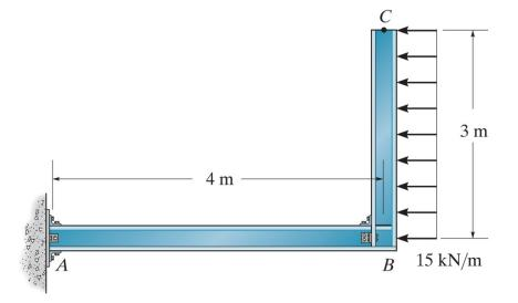
**Example 8c-6**: Compute the vertical displacement at point *C* on the frame shown. Include only the effects of the bending moment in your virtual work equations.
