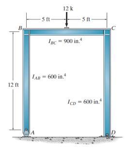
**Example 8c-3**: Determine the slope at point A. Assume E = 29,000 ksi.
