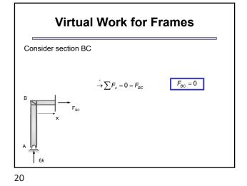
**Virtual Work for Frames** In this problem, the virtual axial forces are the real axial forces divided by 12, based on the principle of superposition. 12 k Section Ν n 8 ft 8 ft D в AB -6k -0.5 BC 0 0 10 ft DC 0 0 DE -6k -0.5
