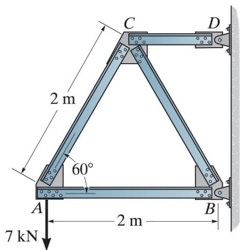
**Example 8a-2:** Determine the vertical displacement of joint A. Assume  $AE$  is constant.
