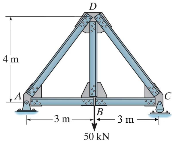
**Example 8a-1:** Determine the vertical displacement of joint *D*. Assume *AE* is constant.
