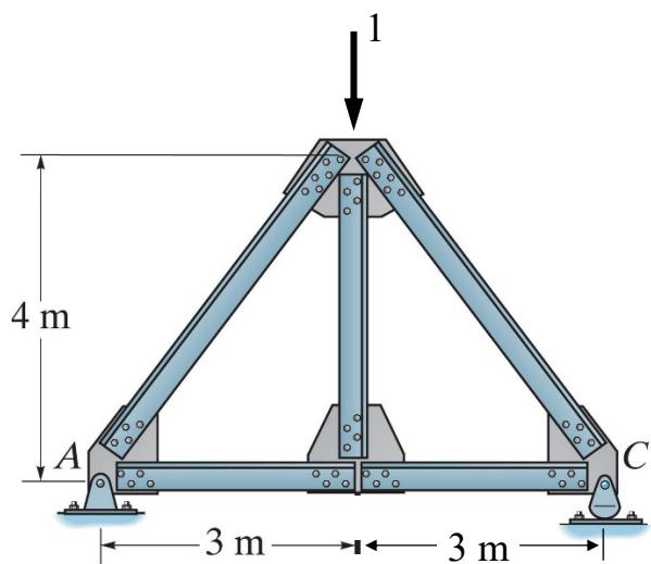
**Example 8a-2:** Determine the vertical displacement of joint A. Assume  $AE$  is constant.
