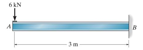
**Example 7a-6:** Determine the equations for slope and displacement in the following beam.
