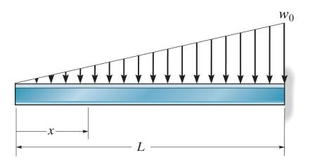
**Example 7a-7:** Determine the equations for slope and displacement in the following beam.
