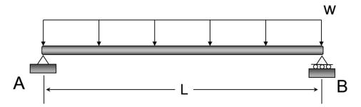
**Example 7a-2:** Determine the equations for slope and displacement in the following beam.
