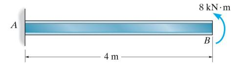
**Example 7a-7:** Determine the equations for slope and displacement in the following beam.
