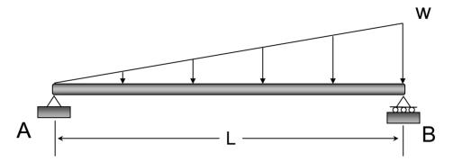
**Example 7a-3:** Determine the equations for slope and displacement in the following beam.
