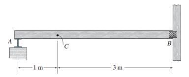
**Example 6b-1**: The beam supports a uniform dead load of 500 N/m and a single live concentrated force of 3 kN. Determine (a) the maximum positive moment at *C* and (b) the maximum positive shear at *C*.
