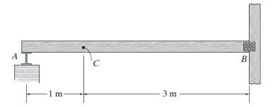
**Example 6b-1**: The beam supports a uniform dead load of 500 N/m and a single live concentrated force of 3 kN. Determine (a) the maximum positive moment at *C* and (b) the maximum positive shear at *C*.
