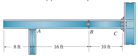
**Example 6b-4**: The beam supports a uniform dead load of 200 lb/ft, a uniform live load of 400 lb/ft, and a single live concentrated force of 10 k. Determine (a) the maximum positive moment at *C* and (b) the maximum positive shear at *B*.
