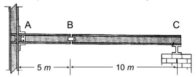
**Example 6a-5**: Determine the maximum *positive* moment that can be developed at point C on the beam shown below due to a single concentrated live load of 8 k, a uniform live load of 3 k/ft., and a beam weight (dead load) of 1 k/ft.
