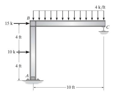
**Example 4d-2**: Draw the shear and moment diagrams for the following frame:
