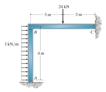
**Example 4d-3**: Draw the shear and moment diagrams for the following frame:
