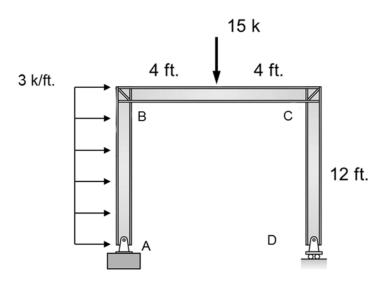
**Example 4d-2**: Draw the shear and moment diagrams for the following frame:
