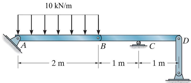
**Example 4c-8** – Construct the shear force and bending moment diagrams.
