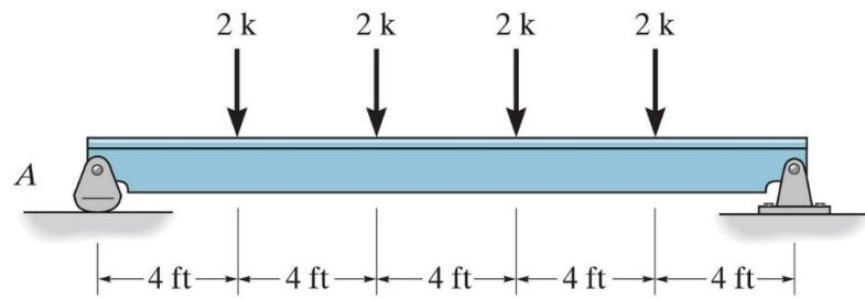
**Example 4c-2** – Construct the shear force and bending moment diagrams.
