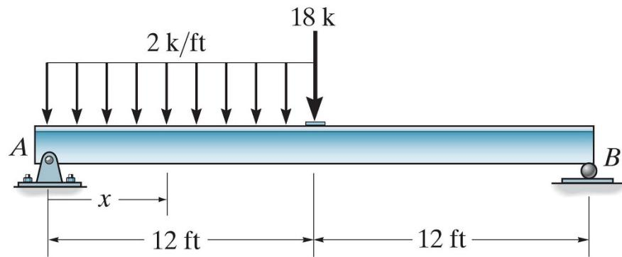
**Example 4c-4** – Construct the shear force and bending moment diagrams.
