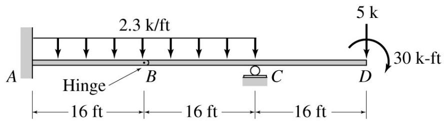
**Example 4c-12 –** Construct the shear force and bending moment diagrams.
