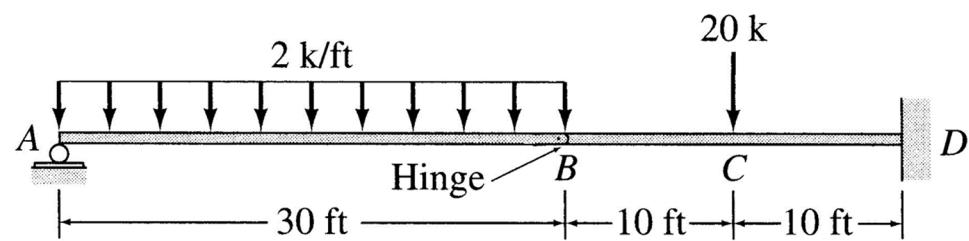
**Example 4c-11** – Construct the shear force and bending moment diagrams.
