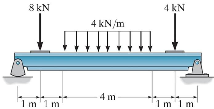
**Example 4c-8** – Construct the shear force and bending moment diagrams.
