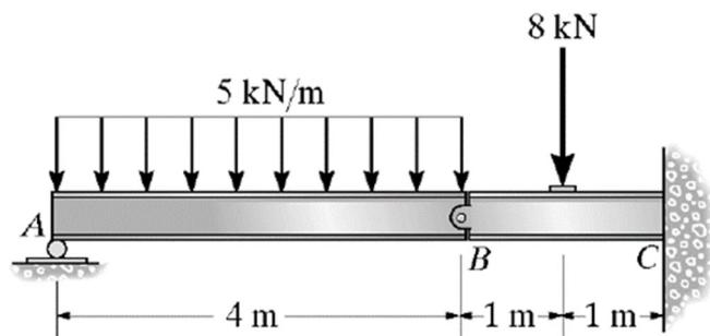
**Example 4c-9** – Construct the shear force and bending moment diagrams.
