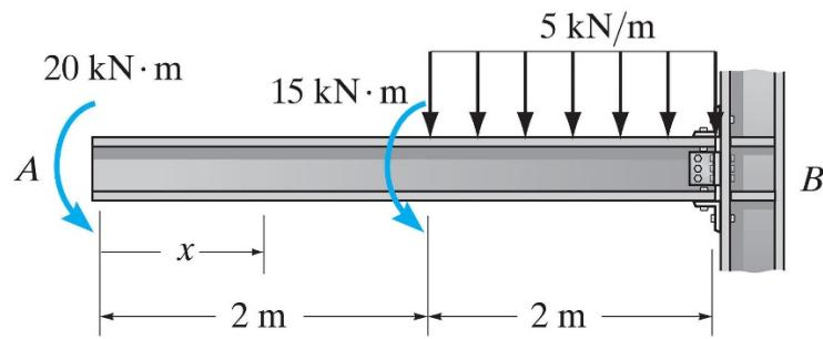
**Example 4c-6** – Construct the shear force and bending moment diagrams.
