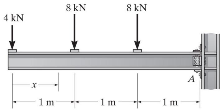
**Example 4c-3 – Construct the shear force and bending moment diagrams.**
