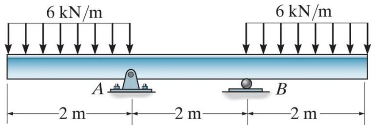
**Example 4c-7 – Construct the shear force and bending moment diagrams.**
