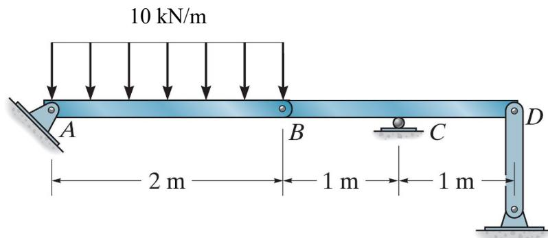
**Example 4c-9** – Construct the shear force and bending moment diagrams.
