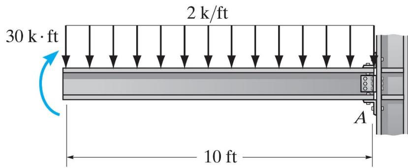
**Example 4c-5 – Construct the shear force and bending moment diagrams.**
