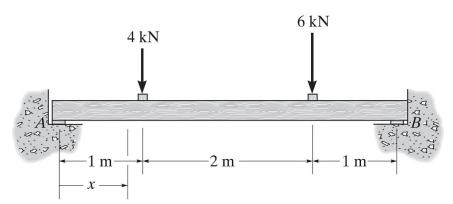
**Example 4b-8** - Determine the internal shear and bending moment as a function of *x*.
