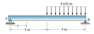
**Example 4b-6** - Determine the internal shear and bending moment as a function of *x*.
