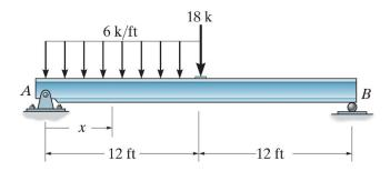
**Example 4b-7** - Determine the internal shear and bending moment as a function of *x*.
