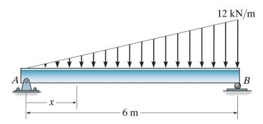
**Example 4b-8** - Determine the internal shear and bending moment as a function of *x*.
