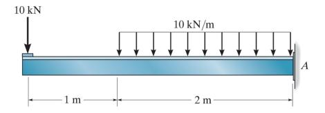
**Example 4b-4** - Determine the internal shear and bending moment as a function of *x*.
