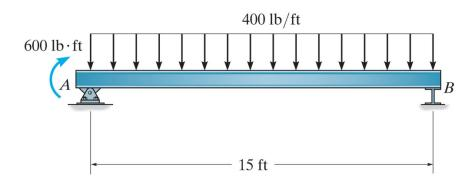
**Example 4b-3** - Determine the internal shear and bending moment as a function of *x*.
