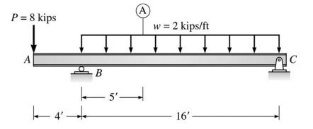
**Example 4b-5** - Determine the internal shear and bending moment as a function of *x*.
