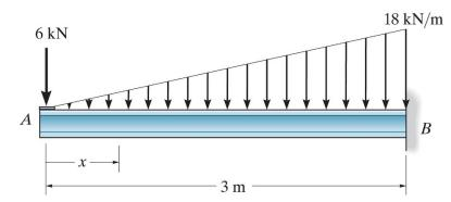
**Example 4b-2** - Determine the internal shear and bending moment as a function of *x*.
