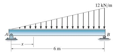
**Example 4b-7** - Determine the internal shear and bending moment as a function of  $\boldsymbol{x}$ .
