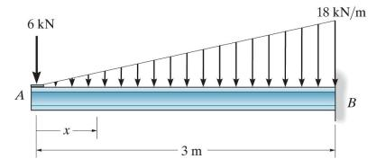
**Example 4b-6** - Determine the internal shear and bending moment as a function of  $\boldsymbol{x}$ .
