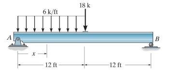
**Example 4b-9** - Determine the internal shear and bending moment as a function of  $\boldsymbol{x}$ .
