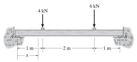
**Example 4b-9** - Determine the internal shear and bending moment as a function of  $\boldsymbol{x}$ .
