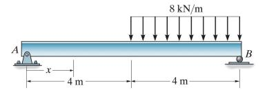
**Example 4b-8** - Determine the internal shear and bending moment as a function of  $\boldsymbol{x}$ .
