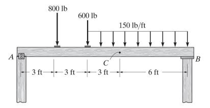
**Example 4a-8** - Determine the internal shear force and bending moment acting at point C.
