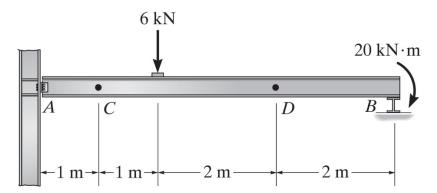
**Example 4a-2** - Determine the internal shear and moment at a section passing through point C.
