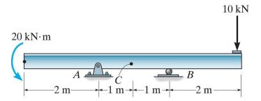
**Example 4a-5** - Determine the internal shear force and bending moment at a section to left of point *D*.
