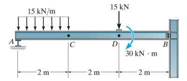
**Example 4a-6** - Determine the internal shear force and bending moment acting at point C.
