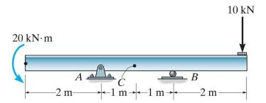
**Example 4a-5** - Determine the internal shear force and bending moment at a section to the left of point *D*.
