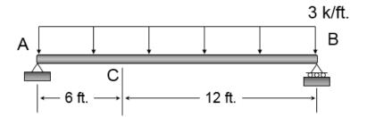
**Example 4a-3** - Determine the internal shear and moment at a section passing through point C.
