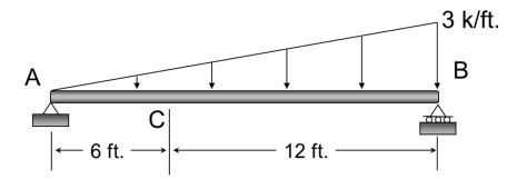
**Example 4a-4** - Determine the internal shear and moment at a section passing through point *C*.
