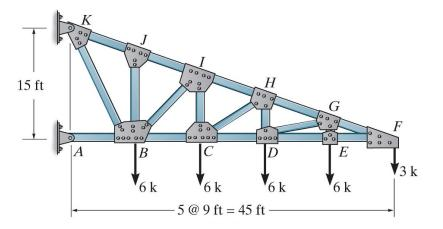
Example 3c-6: Determine the forces in all bars of the truss
