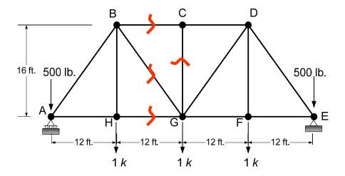
**Example 3c-2:** Determine the forces BC, CG, and GF in the following truss.
