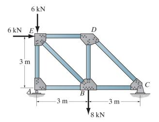
**Problem 3c-7:** Determine the forces in all bars of the truss.
