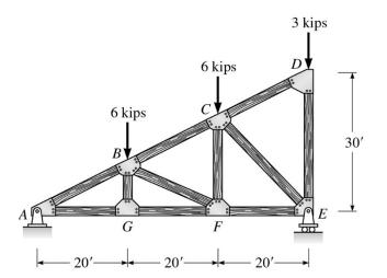
**Problem 3c-7:** Determine the forces in all bars of the truss.
