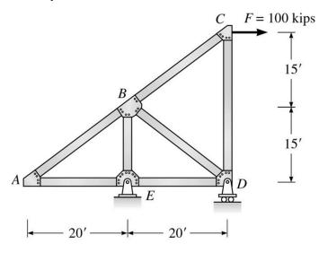
**Example 3b-3**. Determine all the forces in the following truss.
