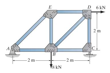
Example 3b-4. Determine all the forces in the following truss.
