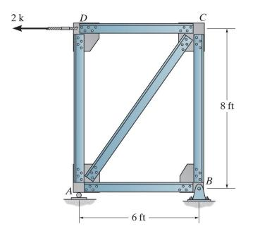
**Example 3b-2**. Determine all the forces in the following truss.
