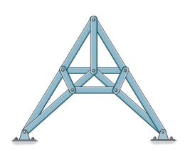
**Example 3a-2**. Classify each truss as determinate, indeterminate, or unstable.
