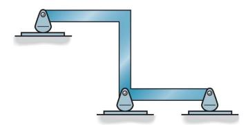
**Example 2b-2**: Classify each structure as determinate, indeterminate, or unstable.
