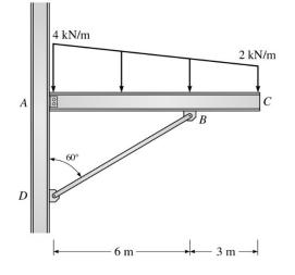
**Problem 2a-4** - Determine the horizontal and vertical reactions at *A* and *C* of the two-member frame.
