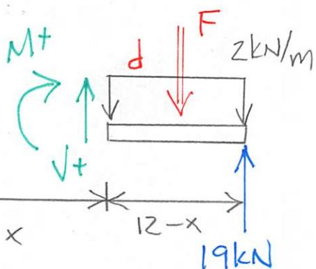
$$\begin{aligned} \sum M_{\text{cut}} &= 0 = -M - 2(12-x)\frac{12-x}{2} \\ &+ 19(12-x) \end{aligned}$$
