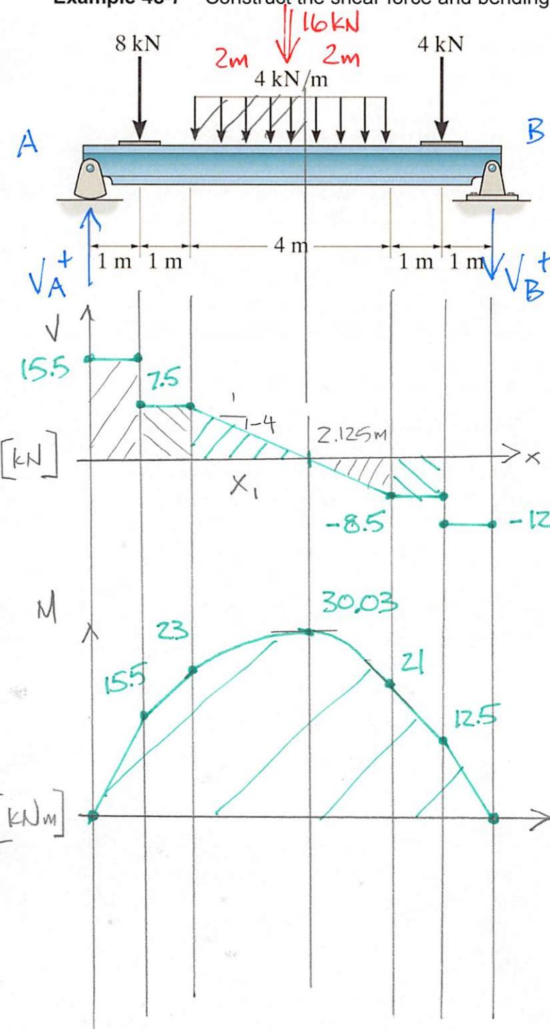
$$\text{At } \sum M_B = 0 = 4\text{kN}(1\text{m}) + 16\text{kN}(4\text{m}) + 8\text{kN}(7\text{m}) - V_A(8\text{m})$$
