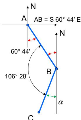
$$\begin{aligned} \alpha &= 179^\circ 60' \\ &\quad - 60^\circ 44' \\ &\quad - 106^\circ 28' \\ \hline & 12^\circ 48' \end{aligned}$$
