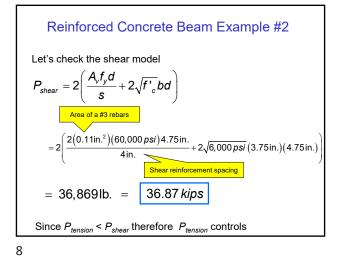
Reinforced Concrete Beam Example #2
