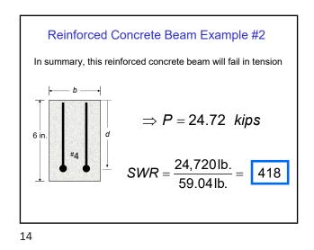
Reinforced Concrete Beam Example #2
