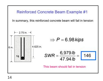
Reinforced Concrete Beam Example #1 The cost of steel may be estimated as follows:  $Cost \text{ of steel} = \frac{A_s L}{1,728 \text{ in}^3/\text{ft}^3} \left( 490 \frac{\text{lb.}}{\text{ft}^3} \right) \left( \frac{\$700}{\text{ton}} \right) \left( \frac{\text{ton}}{2,000 \text{ lb.}} \right)$ where  $A_s$  is the cross-sectional area of steel rebars, L is the length of the steel rebars, and 490 lb./ft.<sup>3</sup> is the unit weight of steel.
