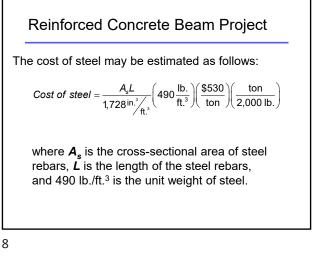
**Reinforced Concrete Beam Project** For example, if one #5 rebar in placed in the beam the steel cost is estimated as:
