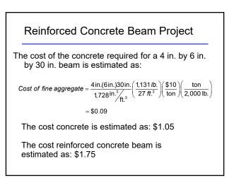
Reinforced Concrete Beam ProjectThe cost adjustment for the reinforced concrete
