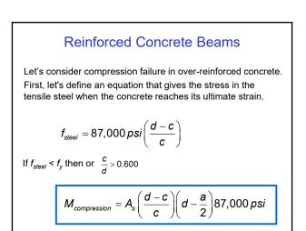
Let's consider compression failure in over-reinforced concrete. First, let's define an equation that gives the stress in the tensile steel when the concrete reaches its ultimate strain.
