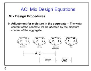
Mix Design Procedures 9. Adjustment for moisture in the aggregate -- The water content of the concrete will be affected by the moisture content of the aggregate.  $\overbrace{Oven dry}$   $\overbrace{Air dry}$   $\overbrace{Sutrated}$   $\overbrace{Wet}$   $\bigvee_{Wet}$ Moisture content (MC) = AC + SM
