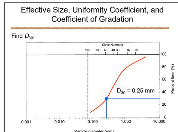
Effective Size, Uniformity Coefficient, and Coefficient of Gradation
