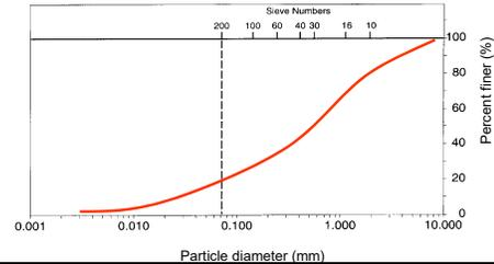
Effective Size, Uniformity Coefficient, and Coefficient of Gradation
