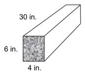
Include a "make-sure-you-have-enough" factor of 1.5 in your mix calculations. Assume a w/c ratio of 0.4 and a mix design of 1:1.5:2. Assume that concrete weighs 145 lb./ft.3. All weights should be reported in 0.05 lb. increments (the precision of the scale in lab).
