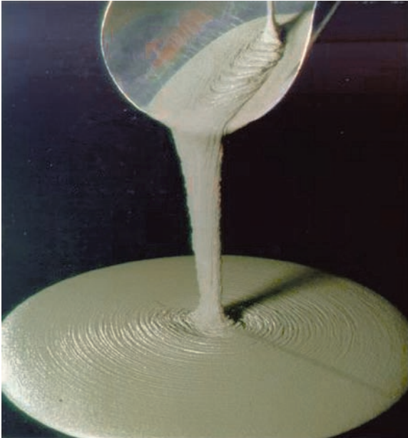
Figure 19-9. Freshly-mixed ultra-high performance concrete.
