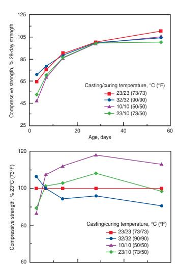
Fig. 12-3. Effect of curing temperature on strength gain (top) relative to 28-day strength and (bottom) relative to the strength of concrete at 23°C (73°F) (Burg 1996).
