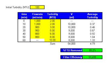
25. If the average turbidity is 10 NTU at the end of 60 minutes, which of the following values most closely estimates the %NTU removed?
